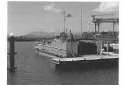
3. The craft starboard side alongside Ross Island wharf with stern loading ramp down.
