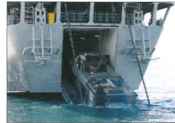
42 Tp LARC V operators conducting stern door marriages with HMAS TOBRUK off the coast of Townsville.
