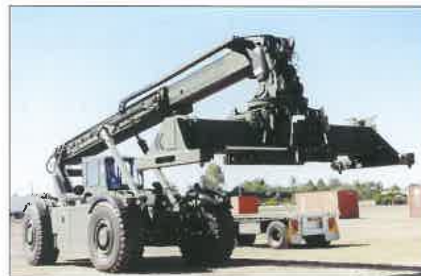
Kalmar with the boom at maximum extension with the top handler in the 40" position.
