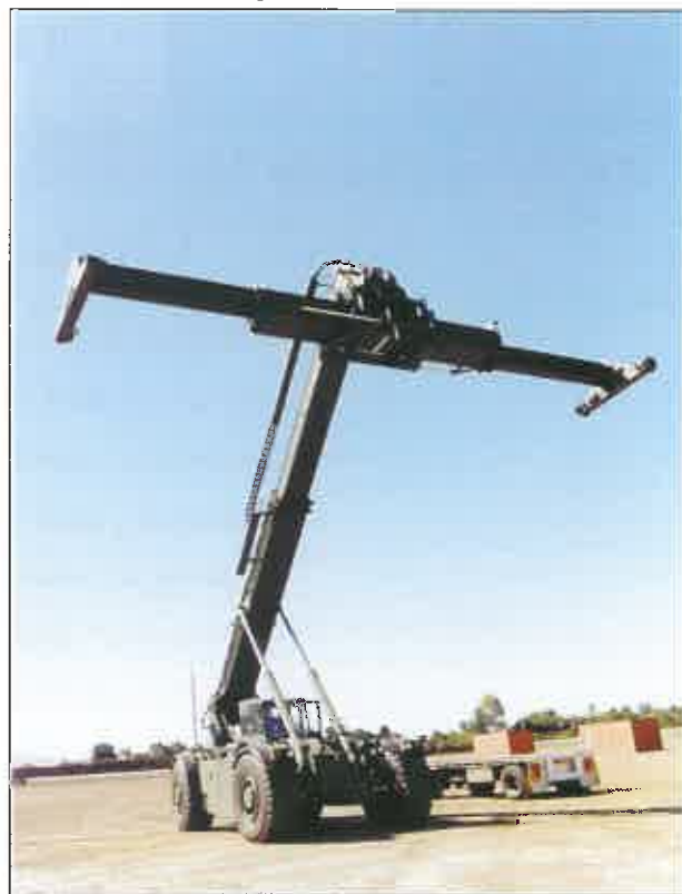
Kalmar lowering boom into the travel position with the top handler in the 20" position
