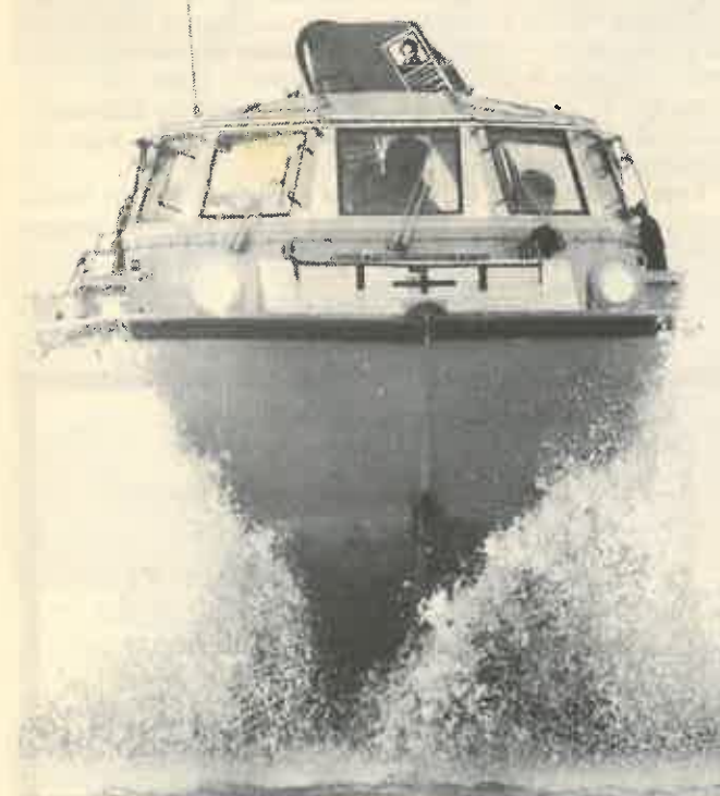
They take to it like a LARC takes to water! A LARC 5, specially modified for work in the Antarctic, emerges from the sea. Its wheels are hidden by the spray.
