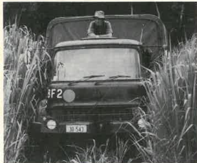
The Bedford MKP lugs through deep, slippery mud on Army trials near Tully, northern Queensland.
