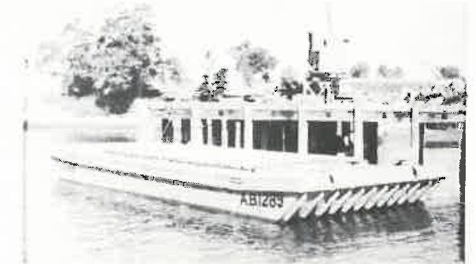
The unit's 60' Philippines Lighter, at Colmslie. The equipment had a removable hatch to allow access to the cargo hold.
