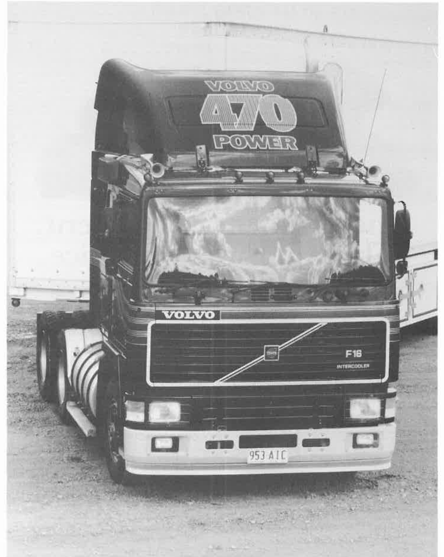
Air shield Kit fitted to Volvo F16 heavy truck (October 1989)
