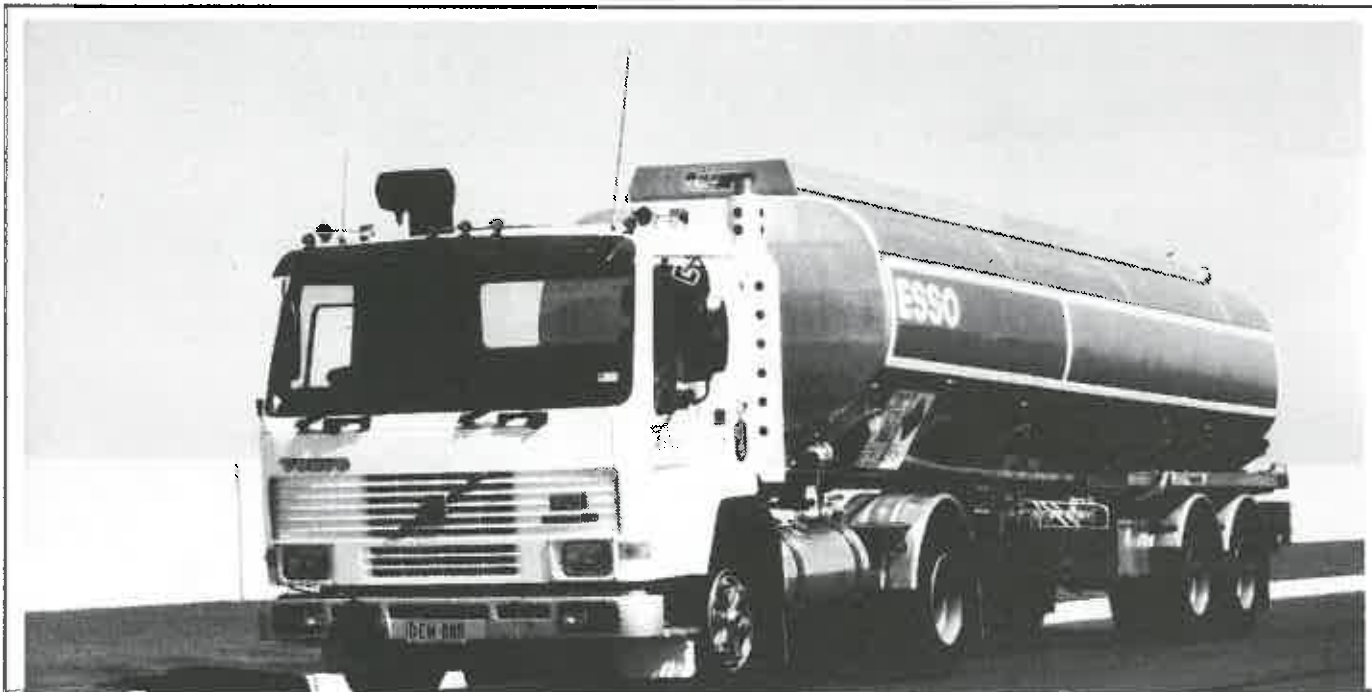
An FL7 as operated by ESSO Australia out of their Botany (NSW) terminal. Unit is a 4 x 2 developing 245 BHP. This is one of several test units that had been operating under Australian conditions since early 1986.
