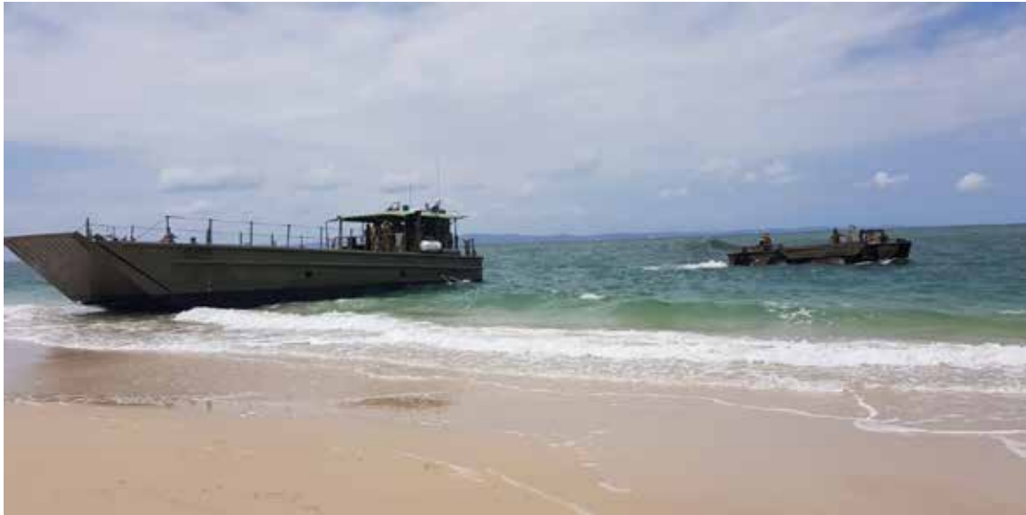
Exercise Surfing Penguin focused on developing skills to operate in high surf conditions. This photo shows LARCs recovering a beached LCM8 in preparation for tasks at Macquarie Island.
