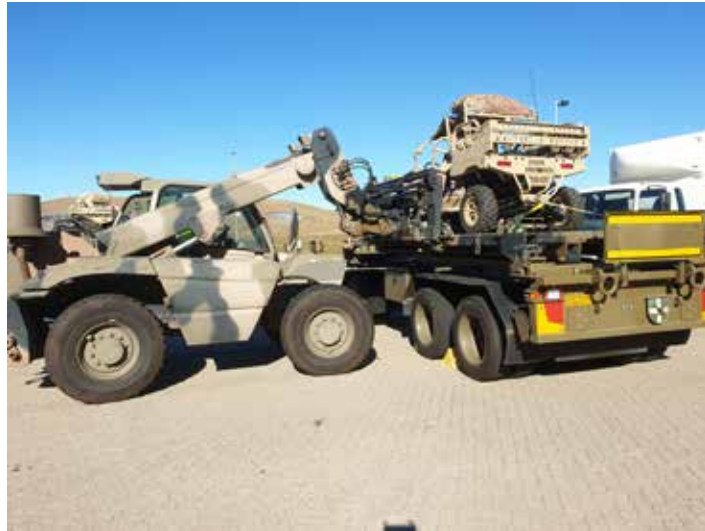
MVT675 Loading Flatrack on ILHS trailer (US RTV)
