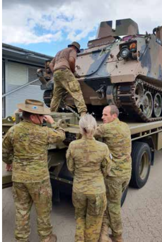
9 TPT SQN drivers conduct training and discussion in methods for restraining loads on the 23t Trailer.
